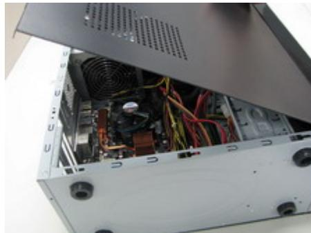
3. Select a PCI Express slot to install the USB 3.0 card into (short and long slots will both work), and remove the metal bracket or placeholder next to the slot.
