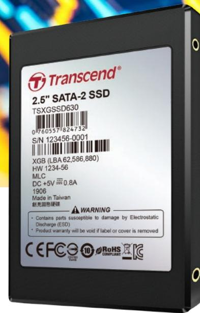
To meet industrial-grade specifications and ensure the utmost quality, Transcend's SSD630 with MLC NAND flash embedded has undergone extensive tests to ensure reliability. Featuring the Advanced Power Shield function, the SSD630 provides extra protection to data integrity against sudden power failures or blackouts, making it ideal for industrial use and mission-critical applications.
